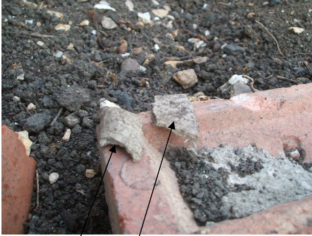
Type 1: Curved or flat cement sheet that is light grey in colour on all sides and edges.
