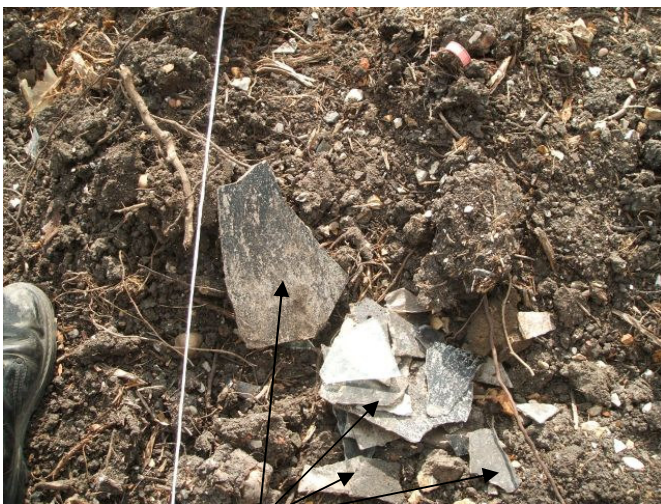
Type 3: Flat cement sheet that is light grey on one side and at the edges and black on the other side.
